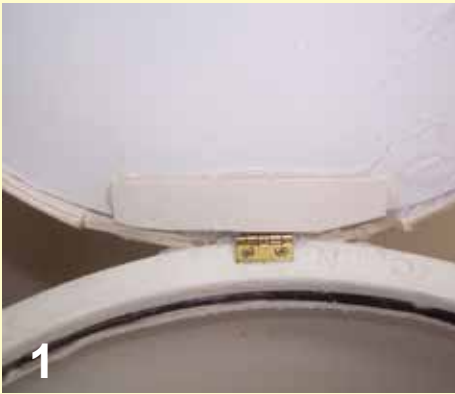
Figures 1 and 2. Note the matting board circles on the bottom side of the top lid. The close-up gives a better view of the hinge itself and where the rim is cut to make room for it. The hinge needs to be on the inside of the bucket for easier opening.
